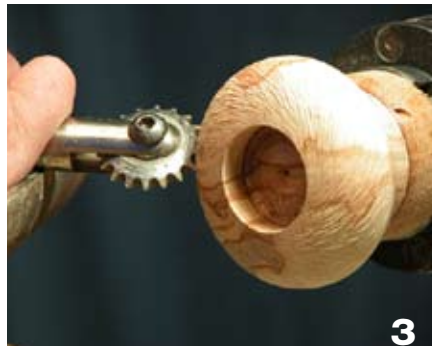
Engage the tool at the edge of the hole and move it toward the edge of the body.
