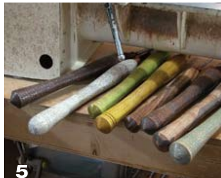
5 With distinctive handles, you'll quickly locate the next tool for your turning task.
